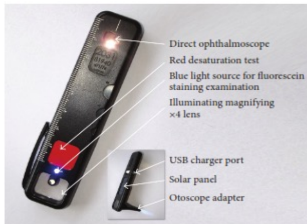
Figure 1: The Arclight direct ophthalmoscope with selected features highlighted. 7
