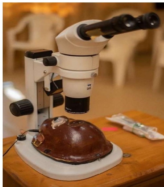
Figure 1: A-P automated Eye Trainer with enucleated animal eyes for surgical training.
